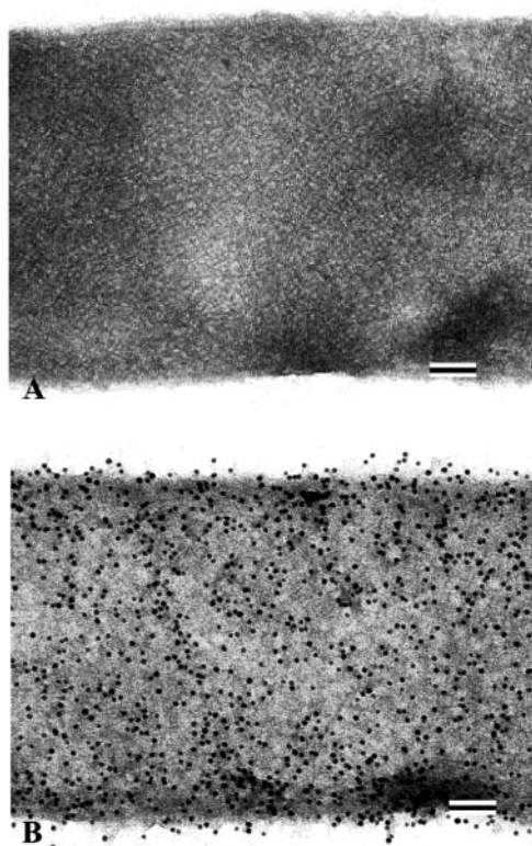
Figure 2. Electron micrographs of negatively stained preparations of recrystallization products formed by rSbpA 31-1068 /cAb-Lys3, (A) before and (B) after binding of anti-camel antibodies and labeling with a Protein A-colloidal gold conjugate. Bars, 100 nm.
